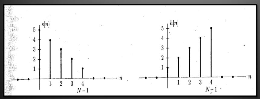
The Matched filter impulse response h(n) is obtained by flipping the signal s(n) about n=0 and shifting to the right by N-1 samples
