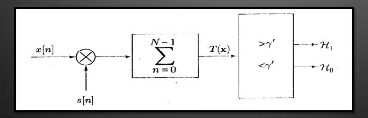
Alternatively we can implement the correlation process using FIR filter which is called Matched filter
