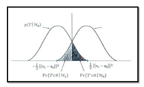
The errors are same because of inherent receiver symmetry
